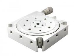
We offer you a fine vacuum compatible rotary stage 860-0140 with a micrometer screw. Stage's motion range is 15° with resolution of 1 arcmin. For coarse adjustment fixing screw can be released and the platform is turned.
